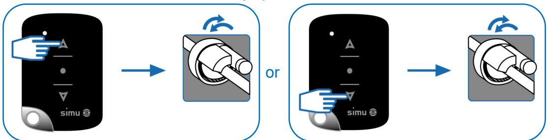
Within 15 seconds, depending on the selected threshold, confirm the settings by pressing the **PROG** key on the transmitter, until the operator responds with a quick, forward and back movement of roughly 1 second.
